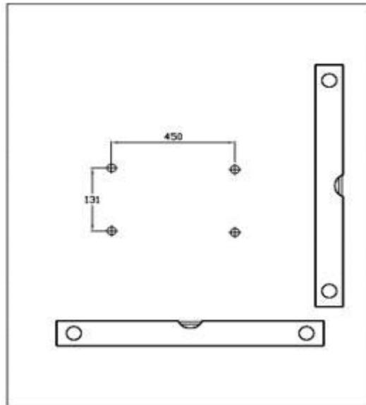
2. Using the drill and 8mm drill bit, drill into the marked positions then insert the wall plugs and tap flush to the finished wall surface.
