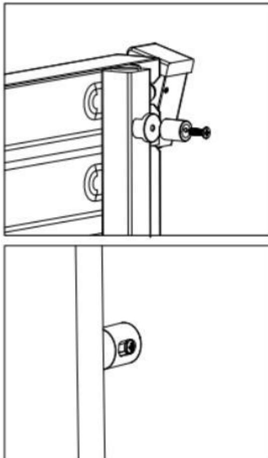
5. Align and push the rail brackets on the radiator onto the wall brackets secured to the wall. Secure the two together with the connecting screws provided (insert through the slot in the bracket) and tighten by the Philips screwdriver, be sure not to overtighten.
